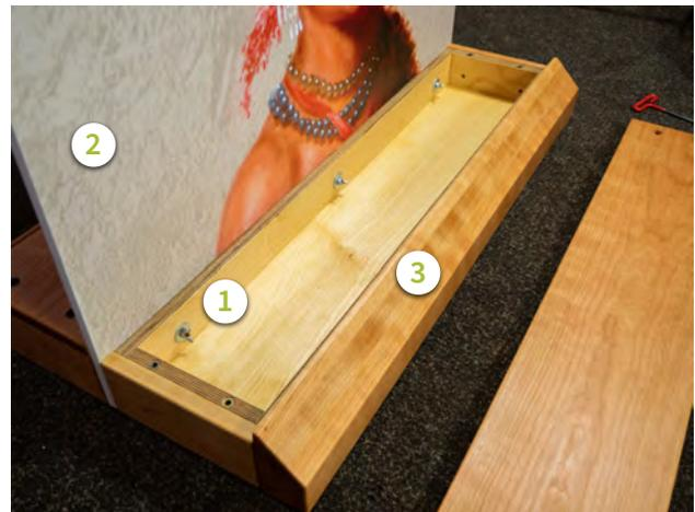
▲ Sign base with the top panel removed to show bolt / wingnut assembly.
